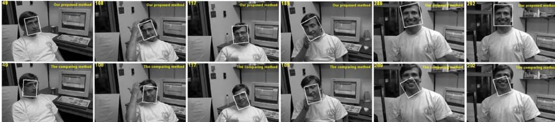
Figure 7. The tracking results of IRSL (row 1) and CTMU (row 2) over representative frames in the scenarios of partial occlusions
