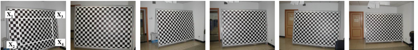
Fig. 4. Images of the calibration board.
