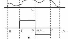
Fig. 2. The bottom row shows the general form of a Haar function \mathbf{v} while the top row is a basis vector \mathbf{u} . The length of \mathbf{v} and \mathbf{u} are both N-1 .
