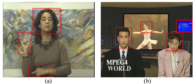
Fig. 1 Some example ROIs in videos (The areas in red rectangles are ROIs).
