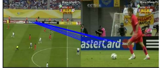
Figure 3: Logo retrieval with partial occlusion and camera motion. Although the logos “MASTERCARD” in the first and second frame have different scales and the second logo is occluded by a people, the frame is included through analyzing the temporal continuity.
