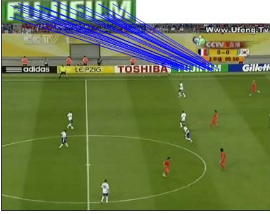
Figure 1: An example of logo descriptors with SIFT features. The image in the left top corner is the logo template, and the bottom is a frame in a video shot. The matched logo descriptors are connected with blue lines.
